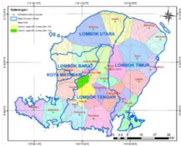
Figure D. Map of Polygon Thiessen Analysis in the Lombok River Basin
