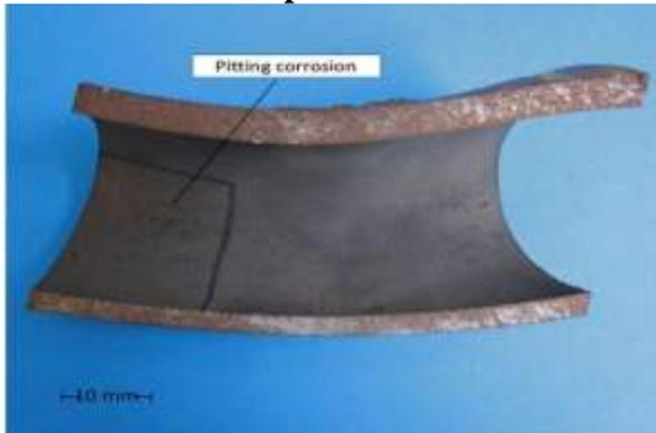
Figure 1. Pitting Corrosion (Duarte et al., 2017)
