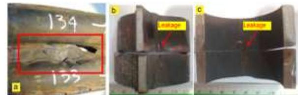
**Figure 7. Visual Inspection of Waterwall Tube Boiler Failure.**
