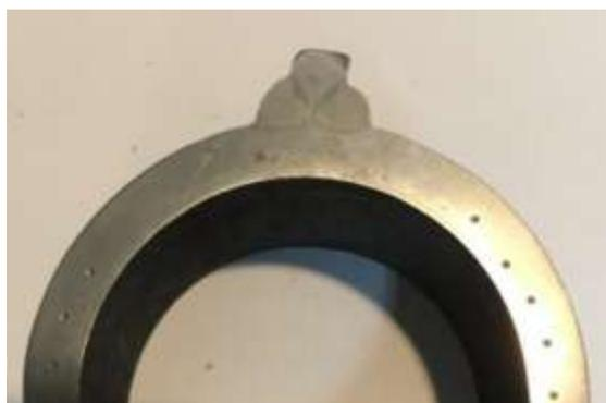
**Figure 13. Waterwall Tube Metallographic Test Specimen 2**
